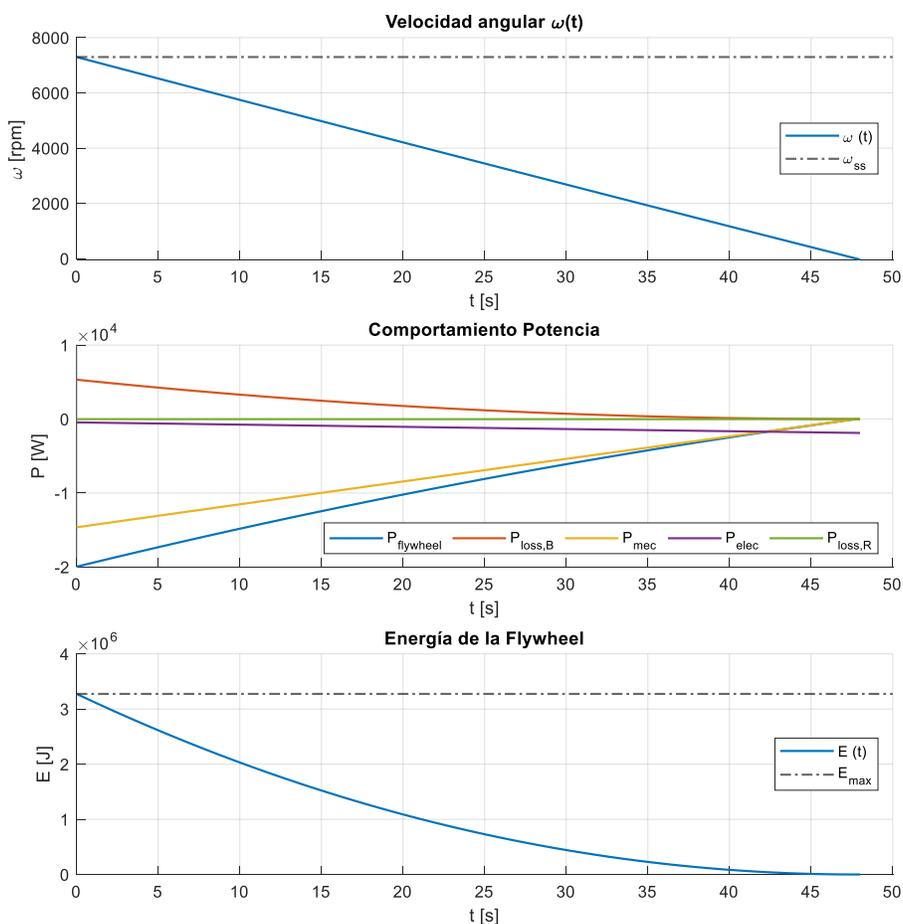
Figura 38. Descarga Flywheel.  $\omega(t)$ ,  $P(t)$ ,  $E(t)$ .  $i_{out} = 30 A$
