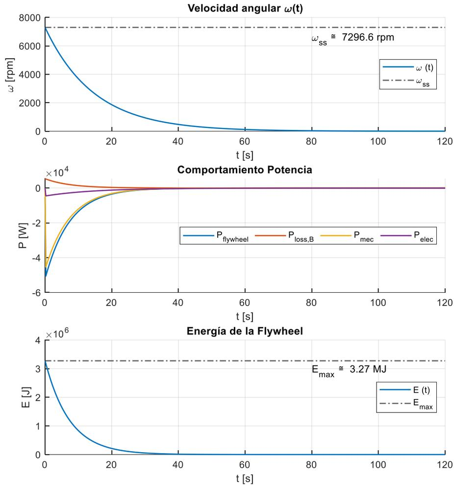
Figura 36. Descarga Flywheel.  $\omega(t)$ ,  $P(t)$ ,  $E(t)$ .  $V_{out} = 48$  V
