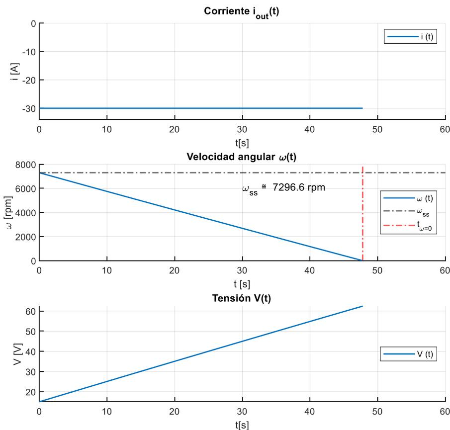
Figura 33. Descarga Flywheel a corriente constante  $i_{out} = 30 A$
